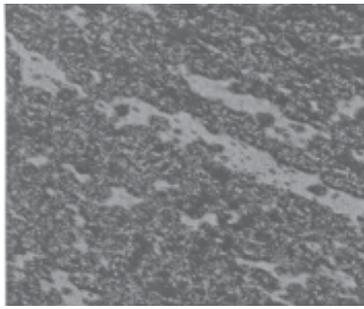
Fig. 9. CoCrMo alloy after homogenization annealing, 320X
