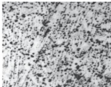
Fig. 3. CoCrMo Alloy - cast condition, heat untreated, 100X, attack solution:  $\text{FeCl}_3$
