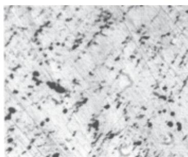
Fig. 5. CoCrMo Alloy - cast condition, heat untreated, 320X, attack solution:  $\text{FeCl}_3$
