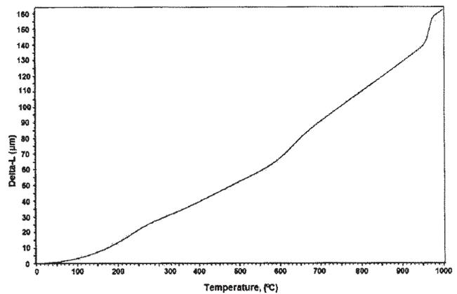
Fig. 12. Variation of temperature coefficient of expansion for CoCrMo alloy, state after homogenization annealing treatment.
