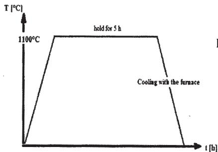
Fig. 2. Heat treatment temperature profile
