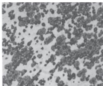
Fig. 8. CoCrMo alloy after homogenization annealing, 200X
