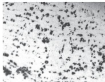
Fig. 4. CoCrMo Alloy - cast condition, heat untreated, 200X, attack solution:  $\text{FeCl}_3$
