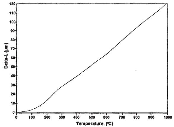
Fig. 11. Variation of temperature coefficient of expansion for CoCrMo alloy, cast condition
