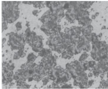
Fig. 10. CoCrMo alloy after homogenization annealing, 500X
