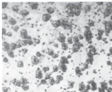
Fig. 7. CoCrMo alloy after homogenization annealing, 100X
